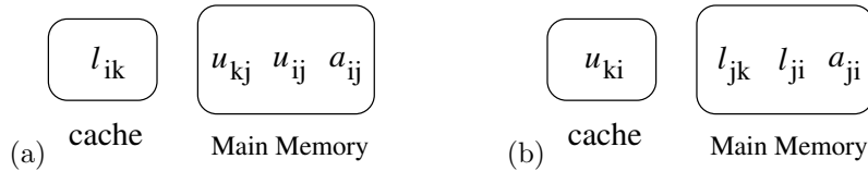
Figure 4.2 Residence of variables in cache and main memory in the compact scheme in the computation of line 1 (a) and line 2 (b) of (4.4).
